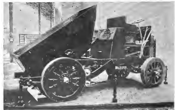
BERNA FOUR-CYLINDER TRUCK WITH PIVOTING BODY.
